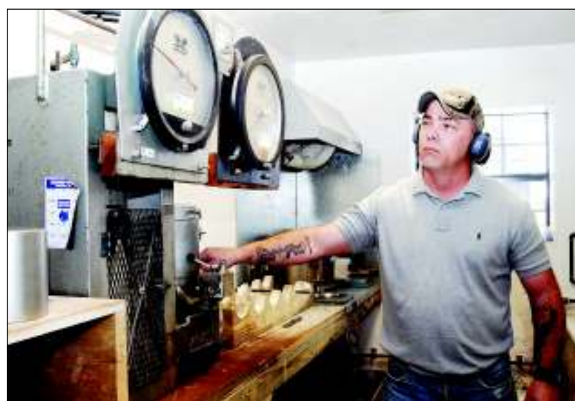
Staff Sgt. James Taylor, WTB, tests the strength of a concrete sample at the Corps of Engineers Quality Assurance Office at Fort Hood. Taylor has been with the agency for more than four months.
