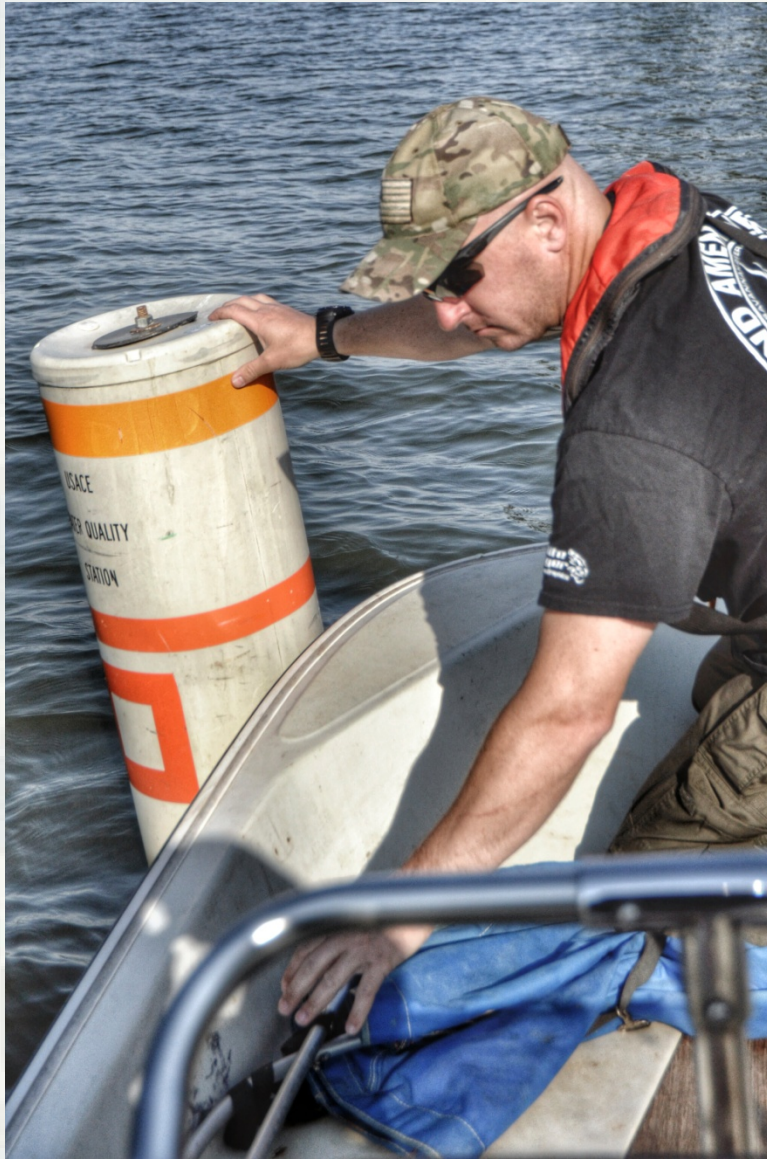
Placing water quality buoys at Thurmond
