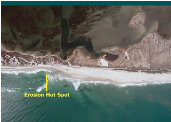
Figure 5. Erosion along the shore can be highly variable, even over short distances, as evidenced by this erosion “hot spot” adjacent to a wide beach. (Photo: Atlantic Coast of New York Monitoring Program, http://dune.seagrant.sunysb.edu/nycoast )
