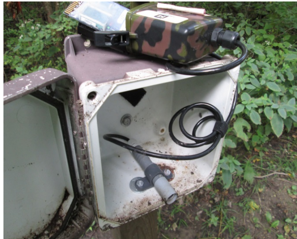
Figure 15 - TRAFx Trail Counter in a fiberglass housing
