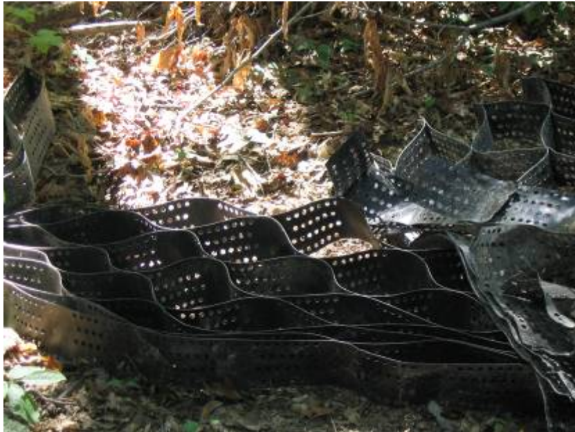
Figure 29. Cave Run Lake, KY. View of geocell – a flexible geosynthetic mat – before placement on the Sheltowee Trace trail for erosion control
