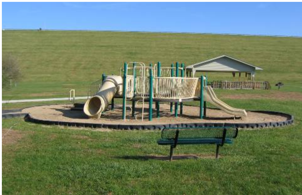
Figure 23. Cave Run Lake, KY. Playground equipment in the COE's Tailwater Recreation Area has a sand-filled impact zone that reduces soils compaction and muddy conditions, and also provides fall-protection for users. Commercially available heavy rubber pads made of shredded tires are provided at selected locations within the impact zone to prevent depressions in the soil that would hold water, and to provide protection in possible fall zones
