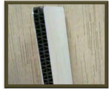
Cross-section example of aluminum-clad corrugated polymer signs.
