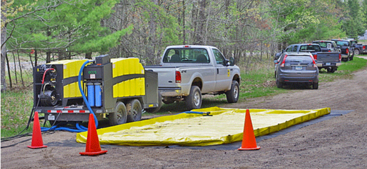
Figure 9. A Portable Decontamination Unit with a Containment Mat for Wastewater
