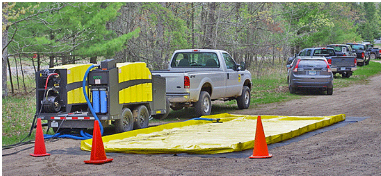
Figure 8. A Portable Decontamination Unit with a Containment Mat for Wastewater
