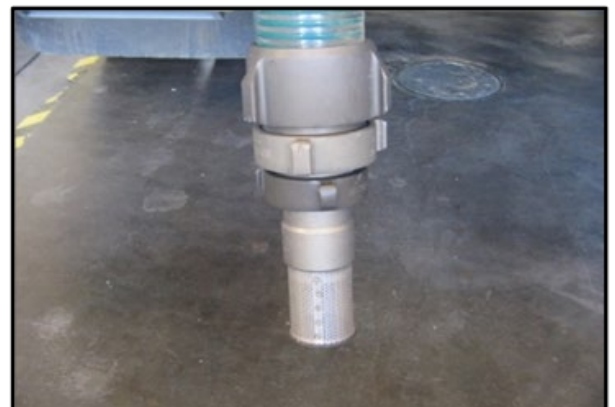
Figure 11: Foot valve attached to suction line with various adapters as needed to adjust for foot valve size
