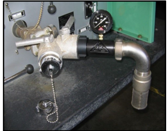
Figure 12: Pressure valve attached to the foot valve
