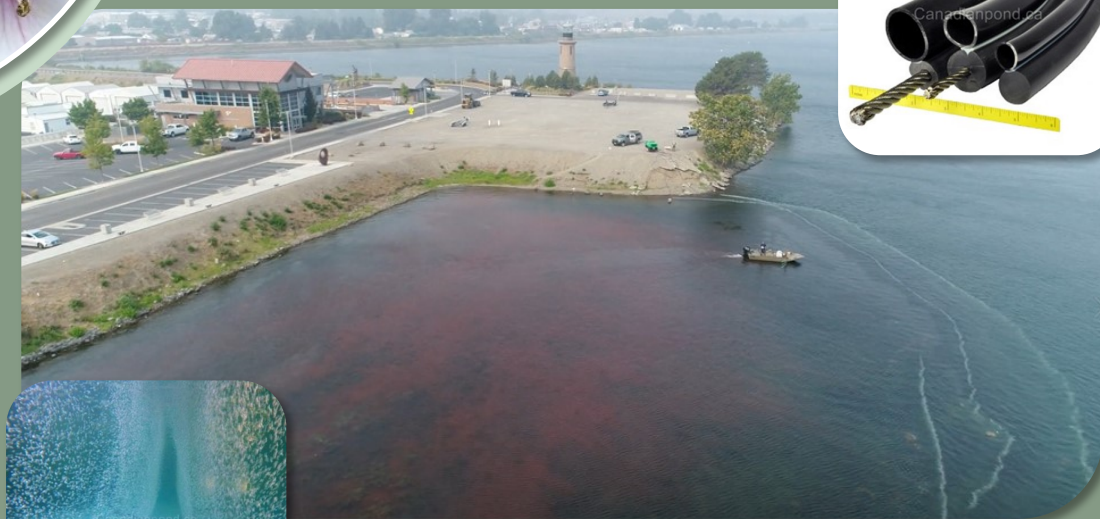
Photo Above: Pictures of bubble curtain post dye treatment to determine water exchange rate. Photos Left and Right: Pictures from manufacturer Canadianpond.ca of the bubble curtain.
