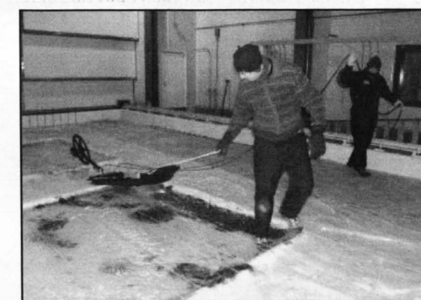
At minus 20 degrees Fahrenheit, a researcher evaluates ground penetrating radar systems to detect oil under and frozen within ice at an ERDC test basin. (Photo courtesy of ERDC)
