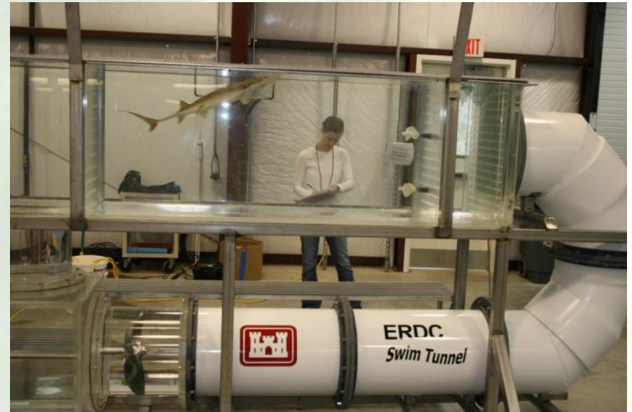
1200 L Tunnel 490 L Working Section
